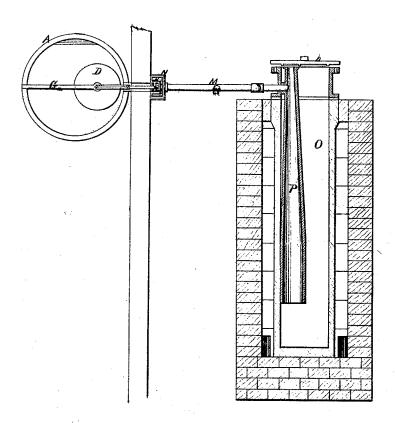
SHOWING RETORT BENCH AND PETROLEUM PIPE IN HORIZONTAL SECTION.
