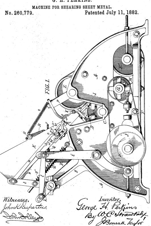
MACHINE FOR SHEARING SHEET METAL.
