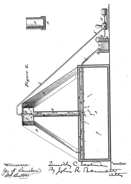
METHOD OF AND APPARATUS FOR COOLING THE AIR IN REFRIGERATING ROOMS.
