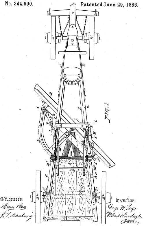
MACHINE FOR MAKING, REPAIRING, AND CLEANING ROADS.
