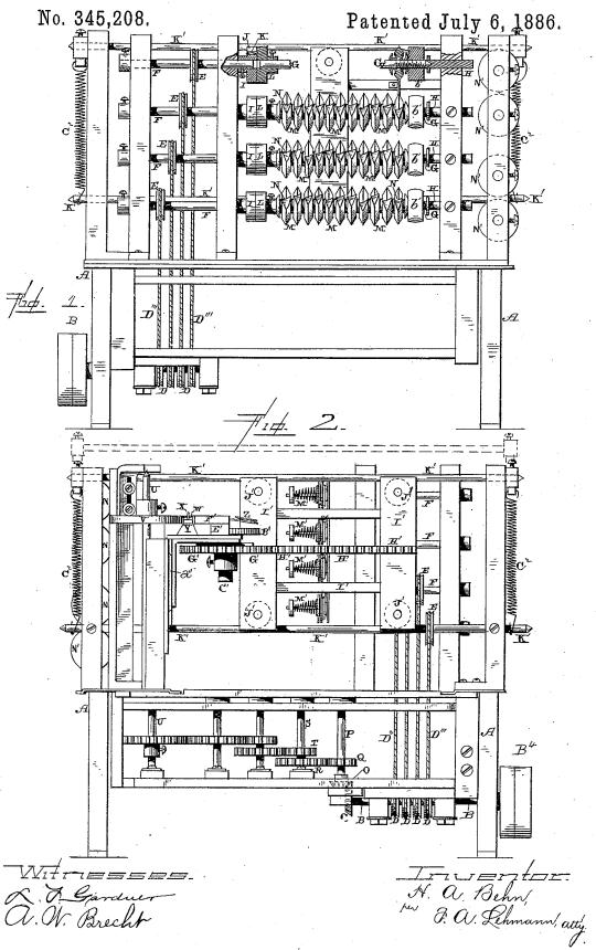
MACHINE FOR WINDING SEWING MACHINE SHUTTLE BOBBINS.
