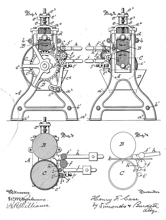
MACHINE FOR SIZING AND COLORING PAPER AND OTHER FABRICS.
