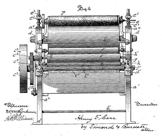
MACHINE FOR SIZING AND COLORING PAPER AND OTHER FABRICS.
