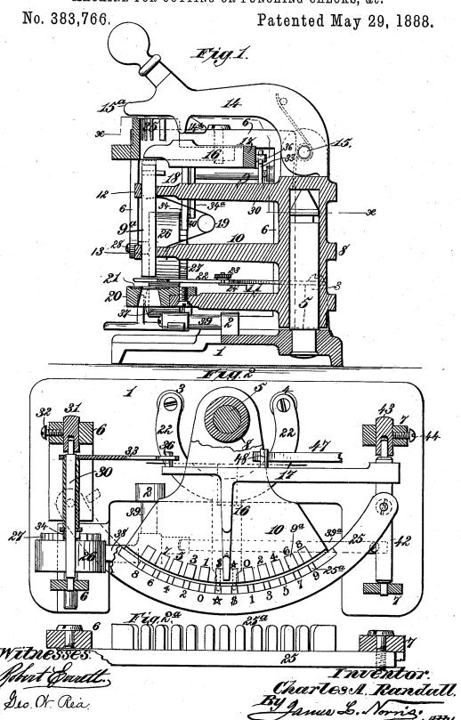
MACHINE FOR CUTTING OR PUNCHING CHECKS, &c.
