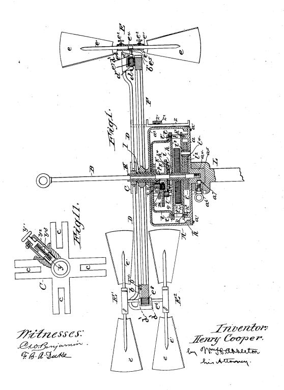
MACHINE FOR AGITATING AND CIRCULATING AIR IN ROOMS, &c. No. 455,660. Patented July 7, 1891.
