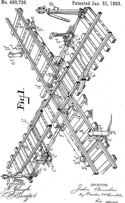
COMBINED SWITCH AND SIGNAL DEVICE FOR RAILWAY CROSSINGS.
