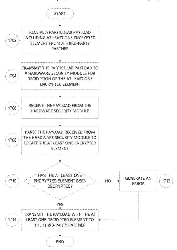
FIG. 17 EXEMPLARY DECRYPTION VERIFICATION PROCESS
