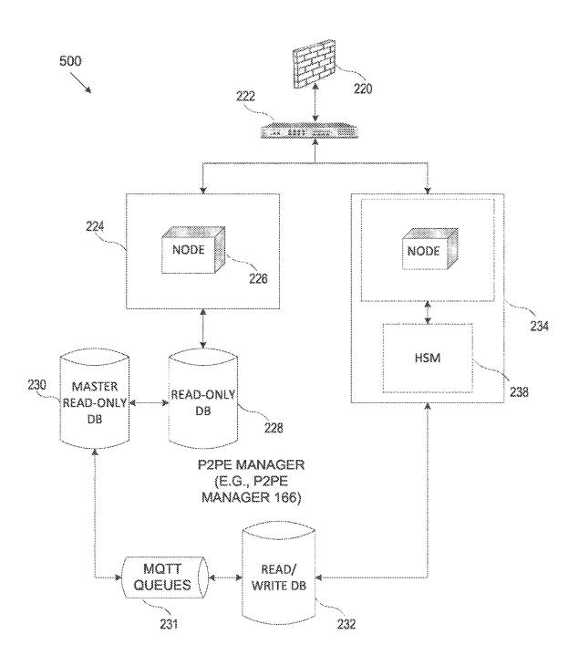
FIG. 2B EXEMPLARY P2PE MANAGER SYSTEM ARCHITECTURE
