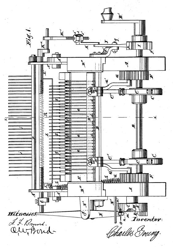
Crocheting-Machine for Making Looped Fabrics.
