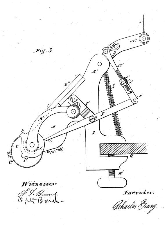
Crocheting-Machine for Making Looped Fabrics.
