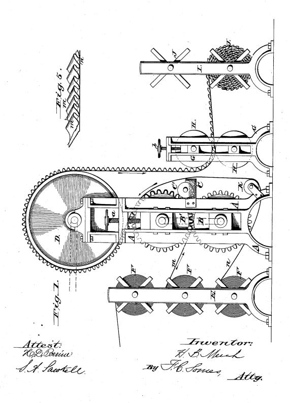
H. B. MEECH. Machine for the Manufacture of Carpet-Lining.
