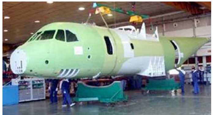
Airframe of first Maritime Patrol Aircraft being manufactured in EADS-CASA facility.
