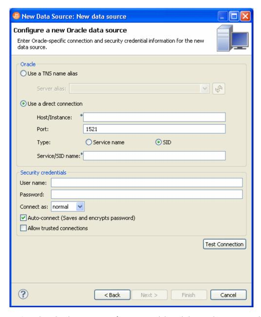
7 Complete the data source configuration and then click **Test Connection**. This will ensure your configuration is correct. If the connection test fails, make the necessary corrections and then click **Finish**.
