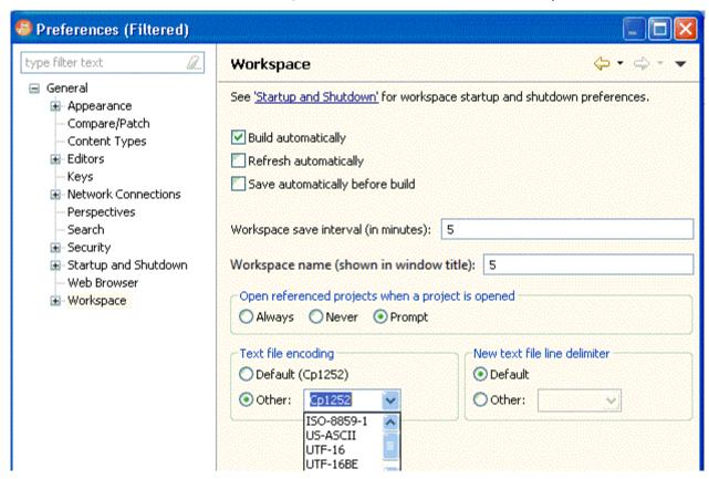
The default encoding for text files on Windows platforms is Cp1252. You can change Unicode support in from file to file using the Text File Encoding options available on the Workspace panel.
