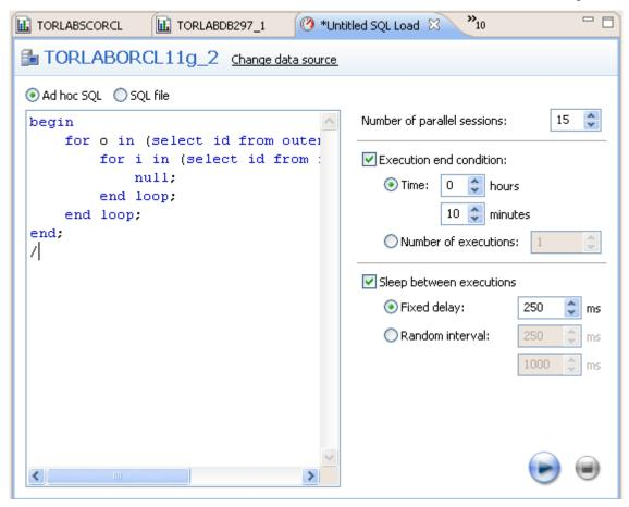
The load editor page has space on the left to show the SQL to be run. The SQL can be typed in or pasted in or read from a file if the **SQL File** option at the top right-hand side of the window is selected.
