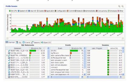
In this case, again the CPU demand is more than the machine can supply but if we look at "Top SQL" we can see that the first SQL statement (with the large green bar) uses up much more CPU than any of the rest, actually 60%! If we could get it down to 10% CPU then we'd save 50% of the CPU usage on the machine! Thus in this case it's worth our while to spend a day or week or even a couple weeks trying to tune that one SQL statement instead of buying a bigger machine.
