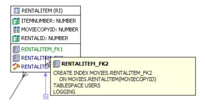
Hovering over the join between two tables displays the relationship between the two tables.
