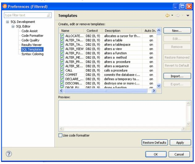
2 Click on the check box beside each template to specify if it is included in the code assist check or not, within SQL Editor. Use the buttons on the right-hand side of the panel to create, edit, or delete SQL templates, as needed.
