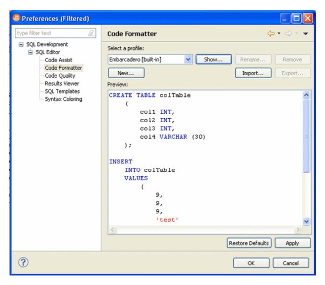
The panel provides a drop down list of formatting profiles and a preview window that displays how each profile formats code.
