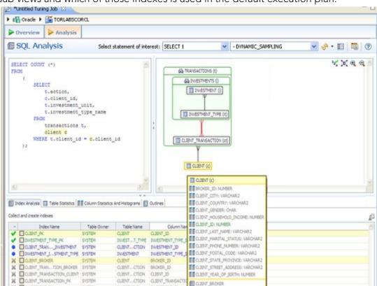
Notice in the view expansion a list of all the indexes on all the underlying tables in the views and sub views and which of those indexes is used in the default execution plan.
