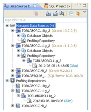
The Profiling Repository entries in the Data Source Explorer are available only when configured in the **Profile Configuration Dialog** for Oracle data sources only. These are saved profiling sessions that you can share with other DB Optimizer users. For information on configuring the data source profiles, see <u>Building Profiling Configurations</u>.
