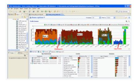
In the above DB Optimizer screen, the same workload was run 4 times. We can see that the time (width of the load) reduced, and the percent of activity on CPU increased.
