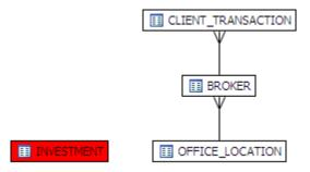
INVESTMENT is highlighted in red with no connectors to indicate that it is joined in via a Cartesian join.
