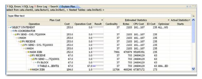
Explain plan operations are shown in a typical tree structure showing parent-child relationships. The following table describes the column groups shown for each operation on the **Explain Plan** tab.
