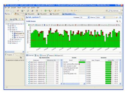
If we look in the bottom left, there is no SQL that takes up a significant amount of load, there is no outlier SQL that we could tune and gain back a lot of wasted CPU. We'd have to tune many SQL and make improvements on most of them to gain back enough CPU to get our load down below the max CPU line. In this case, adding CPUs to the machine might be the easiest and most cost effective solution.
