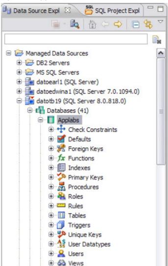
DB Optimizer Object Properties are viewed via the Properties dialog. The dialog is accessed by right-clicking the object in Data Source Explorer.
