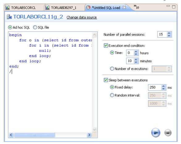
The load editor page has space on the left to show the SQL to be run. The SQL can be typed in or pasted in or read from a file if the **SQL File** option at the top right-hand side of the window is selected.
