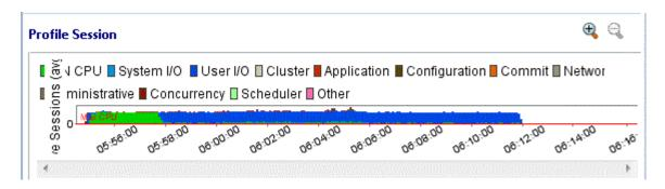
Time is displayed on the X axis, and the Y axis shows the average number of sessions waiting or executing. Each support platform type has a specific set of wait event times. For example, Sybase platforms will display CPU, Lock, Memory, I/O, Network, and Other categories. Use the chart legend to understand the graph. It displays a color and code scheme for executing and waiting session categories in the upper right-hand corner of the chart.
