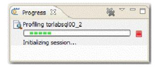
Once a profiling session launches, it runs until you stop it or it has run for its specified length of time. You can stop a session by clicking the **Stop** icon on the right-hand side of the Profiling progress bar.
