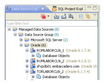
Data Source Explorer sorts databases and database objects by category within DB Optimizer. If data sources are particularly large or complex, or you are only developing specific objects, you can apply database object filters on the view in Data Source Explorer.
