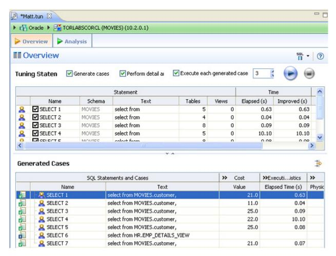
For example, different joining methods such as nested loops or hash joins can be used and will be tested, as appropriate. Tuning will select alternate paths, and enable you to change the original path to one of the alternates. Execution paths slower than the original path are eliminated, which enables you to select the quickest of the returned selections and improve query times, overall.
