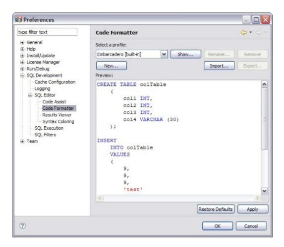
In addition to formatting code per individual file, you can also format an entire group of files from **Project Explorer**. Select the directory of files that you want to apply formatting to and execute the **Format** command from the right-click menu. The files will be automatically formatted based on the global preferences.
