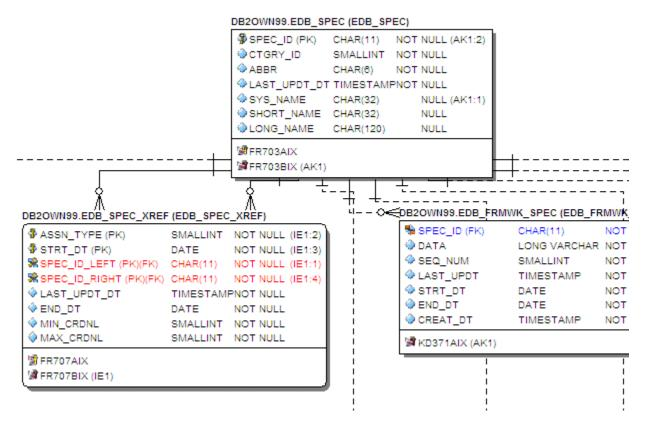
**NOTE:** Since the sizes of the objects changed, you may want to change the model layout using one of the ER/Studio DA advanced layout engines. You can also customize the default display properties for new models by choosing **Tools > Options**, and then selecting the desired options on the **Display** tab.
