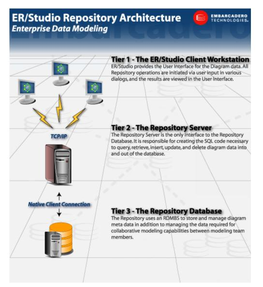
The Repository relies on a native client connection and the TCP/IP protocol to send and receive information between ER/Studio DA, the Repository Server, and the Repository Database. Communications between the client and server are secure. SSL support in the client and repository allows you to specify the common URL and port to support secure communications between the client and the repository.
