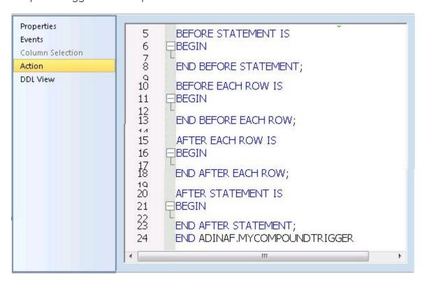
The CREATE OR REPLACE TRIGGER... DDL generated for the trigger built using these options includes the compound trigger-specific FOR clause.
