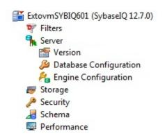
The **Server** subnodes provide access to server, database, and connection properties as well as configuration/initialization parameters.
