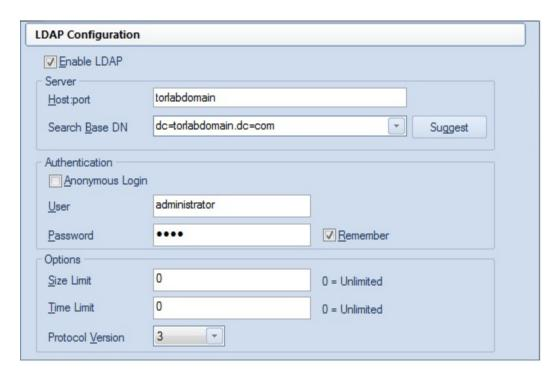
When registering a datasource against one of the supported DBMS platforms, a new **Connection Information** tab control lets you designate the registration as being LDAP-based.
