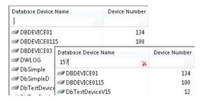
This feature must be enabled. The Options Editor's **Explorer** pane has a **Column filters use regular expressions by default** control that enables regular expression usage when DBArtisan starts or a new Explorer is manually opened.
