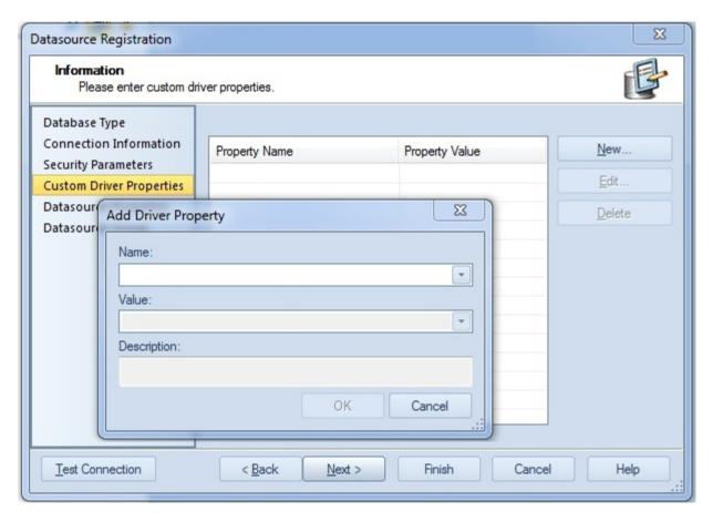
For each platform, all connection string parameters/driver properties supported for that driver can be specified.
