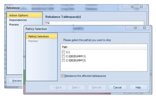
**Rebalance** lets you create containers on recently added storage paths and drop containers from storage paths that are in DROP PENDING state. **Drop Automatic Storage Paths** removes one or more storage paths with an optional REBALANCE operation.
