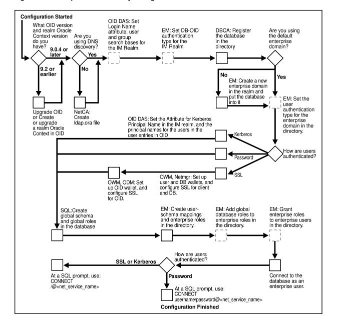
Figure 4-1 Enterprise User Security Configuration Flow Chart
