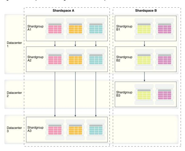
Figure 7-3 Composite Sharding with Data Guard Replication
