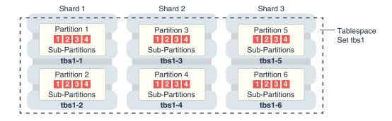
In this example each subpartition is stored in the parent partition's tablespace. Because subpartitioning is done by date, it makes more sense to store subpartitions in separate tablespaces to provide the ability to archive older data or move it to a read-only storage. The appropriate syntax is shown here.
