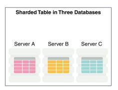
Sharding is based on shared-nothing hardware infrastructure and it eliminates single points of failure because shards do not share physical resources such as CPU, memory, or storage devices. Shards are also loosely coupled in terms of software; they do not run clusterware.
