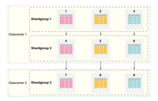
Figure 7-1 System-Managed Sharding with Data Guard Replication
