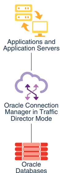
Figure 2-1 Architecture of Oracle Connection Manager in Traffic Director Mode
