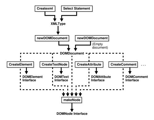
Figure 11-1 Using the PL/SQL DOM API for XMLType
