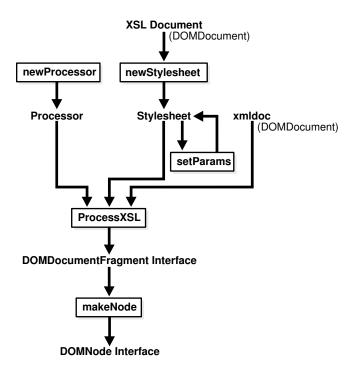
Figure 11-3 Using the PL/SQL XSLT Processor for XMLType
