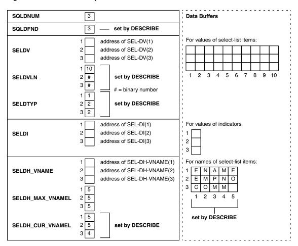
Figure 11-7 Select Descriptor after the DESCR
