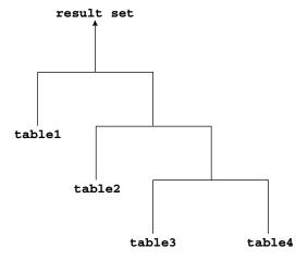
If the left or the right child of an internal node of a join tree can be a join node, then the tree is called a bushy join tree. In the following example, table4 is a right child of a join node, table1 is the left child of a join node, and table2 is the left child of a join node.
