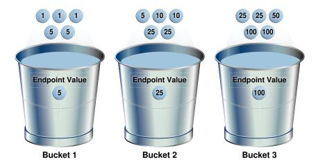
If a bucket border splits a value so that some occurrences of the value are in one bucket and some in another, then the optimizer shifts the bucket border (and all other following bucket borders) forward to include all occurrences of the value. For example, the optimizer shifts value 5 so that it is now wholly in the first bucket, and the value 25 is now wholly in the second bucket.
