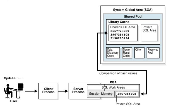
If a check determines that a statement in the shared pool has the same hash value, then the database performs semantic and environment checks to determine whether the statements have the same meaning. Identical syntax is not sufficient. For example, suppose two different users log in to the database and issue the following SQL statements:
