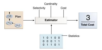
For the query shown in Example 4-1, the estimator uses selectivity, estimated cardinality (a total return of 10 rows), and cost measures to produce its total cost estimate of 3:
