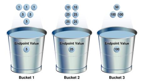
The endpoint repeat count measures the number of times that the corresponding bucket endpoint, which is the value at the right bucket border, repeats itself. For example, in the first bucket, the value 5 is repeated 3 times, so the endpoint repeat count is 3.
