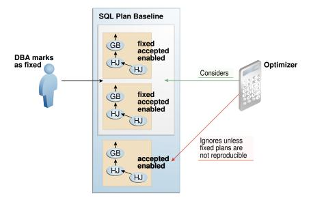
If new plans are added to a baseline that contains at least one enabled fixed plan, then the optimizer cannot use the new plans until you manually declare them as fixed.
