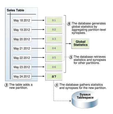
Figure 13-3 Aggregating Statistics after Adding a Partition
