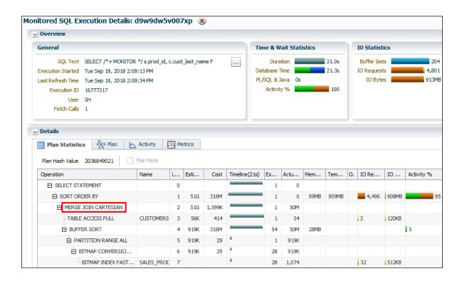
The cause of the performance problem is shown in Line 2: a Cartesian join. The author of the query inadvertently left off the WHERE clause. Instead of returning around 1 million rows as it would for an inner join of sales and customers, the
