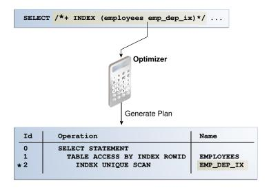
The disadvantage of hints is the extra code to manage, check, and control. Hints were introduced in Oracle7, when users had little recourse if the optimizer generated suboptimal plans. Because changes in the database and host environment can make hints obsolete or have negative consequences, a good practice is to test using hints, but use other techniques to manage execution plans.
