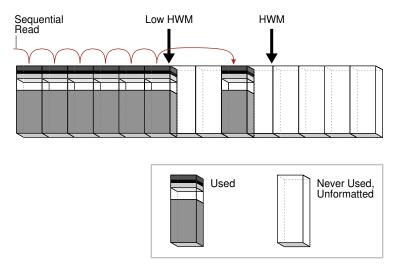
Because the blocks are adjacent, the database can speed up the scan by making I/O calls larger than a single block, known as a multiblock read. The size of
