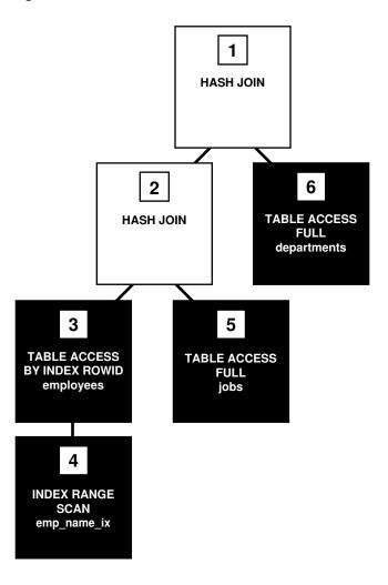
In Figure 3-3, each node of the tree acts as a row source, which means that each step of the execution plan in Example 3-1 either retrieves rows from the database or accepts rows from one or more row sources as input. The SQL engine executes each row source as follows:
