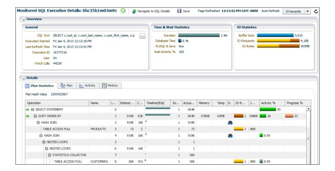
The preceding report shows the execution plan and statistics relating to statement execution. For example, the Timeline column shows when each step of the execution plan was active. Times are shown relative to the beginning and end of the statement execution. The Executions column shows how many times an operation was executed.
