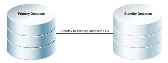
To tune a standby workload on a primary database, specify the <code>database\_link\_to</code> parameter in <code>DBMS\_SQLTUNE</code> procedures. By default, the <code>database\_link\_to</code> parameter is null, which means that tuning is local.
