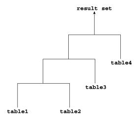
If the left child of every internal node of a join tree is a table, then the tree is called a right deep join tree, as shown in the following diagram.
