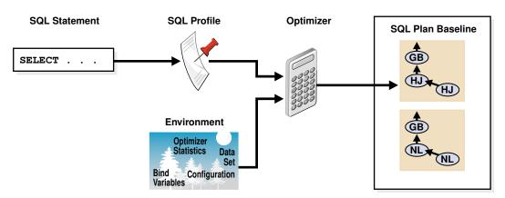
If either the optimizer environment or SQL profile changes, then the optimizer can create a new plan. As tables grow, or as indexes are created or dropped, the plan for a SQL profile can change. The profile continues to be relevant even if the data distribution or access path of the corresponding statement changes.
