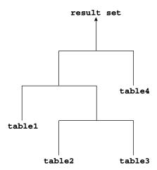
In yet another variation, both inputs of a join are the results of a previous join.
