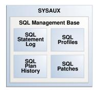
SMB data related to a PDB is stored in the PDB, and is included if the PDB is unplugged. A common user whose current container is the CDB root can view SMB data for PDBs. A user whose current container is a PDB can view the SMB data for the PDB only.
